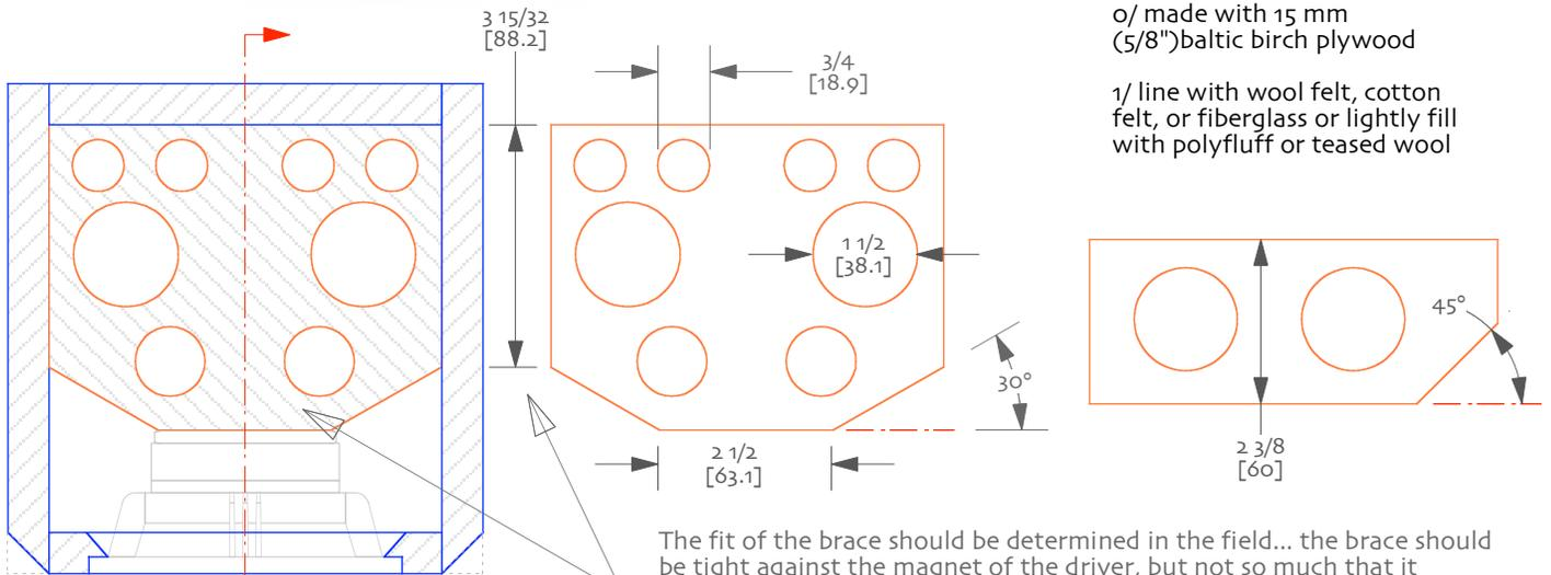
The fit of the brace should be determined in the field... the brace should be tight against the magnet of the driver, but not so much that it stresses the basket... small paper shims can be used if necessary.
